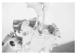
• Align the marks (A) on the camshaft so that they are parallel with the surface of the cylinder head.
