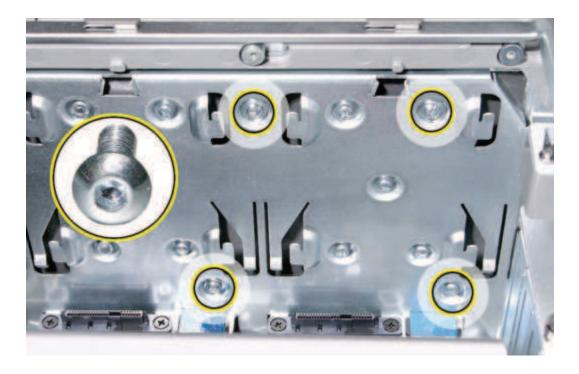
2. Depress the upper right corner of the power supply and slide the power supply toward the front of the computer.
