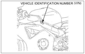
(3) The Vehicle Identification Number (VIN) is located on left side of the main frame on the Safety Certification Labels.
