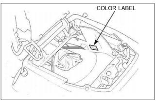
(5) The color label is attached as shown. When ordering color-coded parts, always specify the designated color code.
