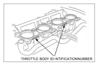
(4) The throttle body identification number is stamped on the intake side of the throttle body as shown.
