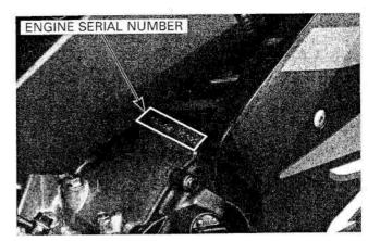
(2) The engine serial number is stamped on the right side of the upper crankcase.
