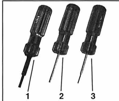
1. Amphenol insert tool 000798 P/N 322697 2. Amphenol pin removal tool P/N 322698 3. Amphenol socket removal tool P/N 322699
